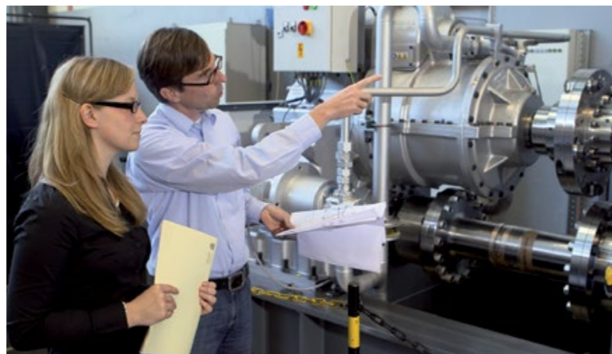
Back-to-back testing of a T 2 RECS 560 LL
