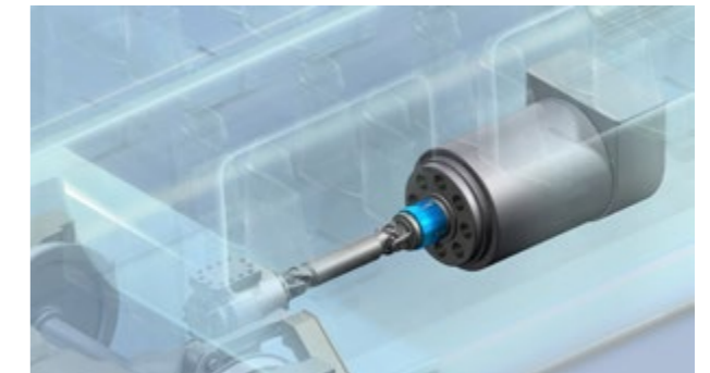
Drive unit of a high-speed train
