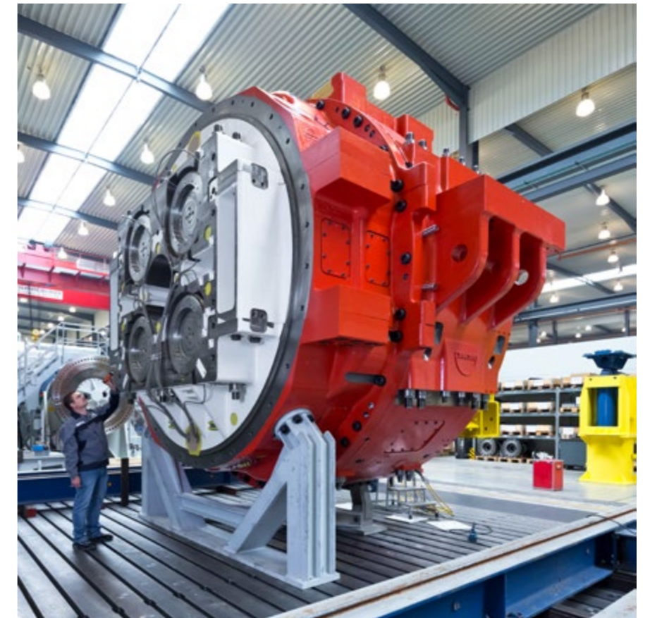
Assembling the world's biggest planetary gear system designed for the megasized wind energy nacelle testing unit at Clemson University, USA. The picture above shows the four planetary stages.
